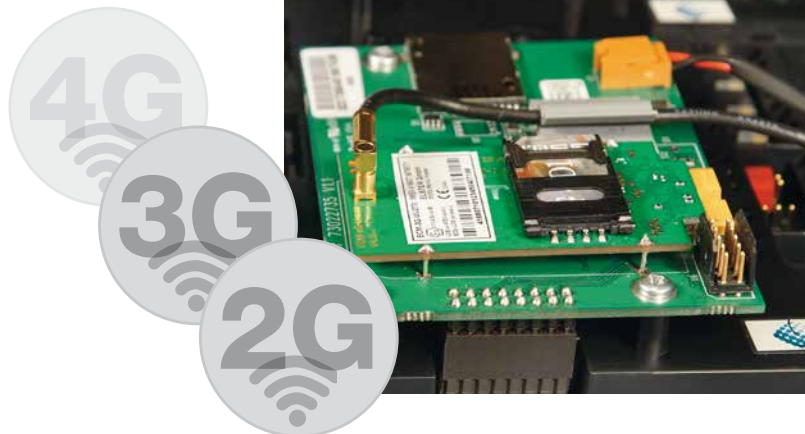
New Modem Module ECM-3G in the EK280
