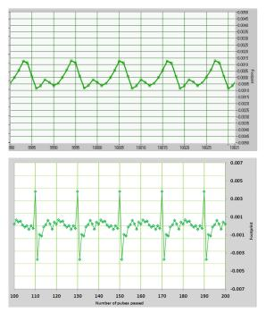
Footprint analysis of undamaged (top) vs. damaged (bottom) rotor
