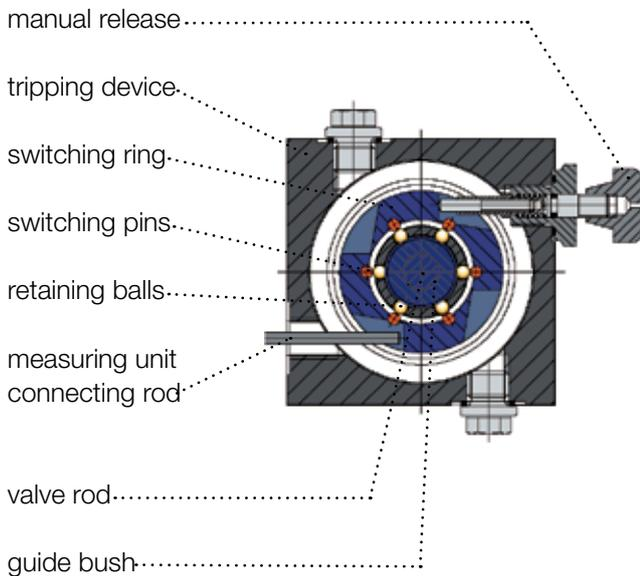
**ball-and-pin tripping device
